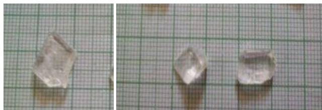
Fig (1). As grown KHP crystals (a). Undoped (b). 0.09mol% (c). 0.15 mol% doped L-Phenylalanine crystals.
